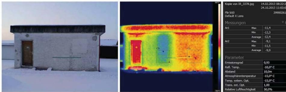
FIG 5. Exterior view of the north side of the test building with IR image, before sunrise, 14<sup>th</sup> Feb 2013. The temperature measured with IR correspond to the measurement with calibrated PT 100 temperature sensor within the accuracy of the measurements.
