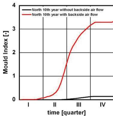
FIG 8. Sequence of the mould-indexes in the interstitial layer between original plaster and new applied adhesive mat calculated with tight and leaky construction on a north oriented facade of the last calculated year.
